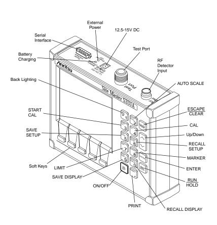
Figure 2-1. Site Master Controls and Connectors
