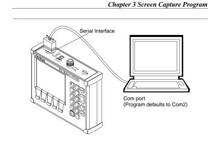
Figure 3-3. Equipment Setup for Site Master Tools Operation
