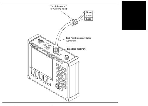
Figure 2-9. Measurement/Calibration Test Setup
