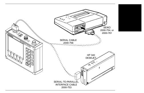
Figure 2-11. Printer Setup
