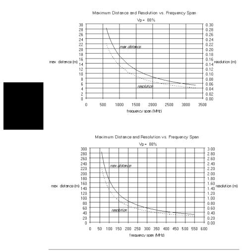
Figure 2-10. Maximum Distance and Resolution vs Frequency Span
